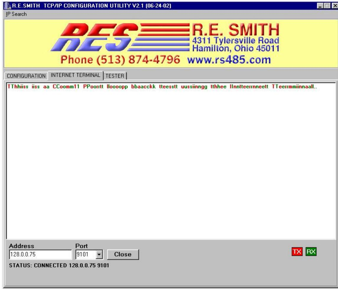
6. To send data on the network to the ESPSX3's COM1, type in the main window of the Configuration Utility's Internet Terminal. The message you type will display in red. The message also appears in green in the I/O Commander's Terminal Emulator window.
